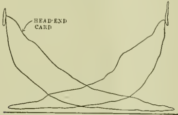
FIG. 6.—INDICATOR CARD TAKEN WHILE LOCOMOTIVE WAS RUNNING AT A SPEED OF 60.5 MILES PER HOUR.
